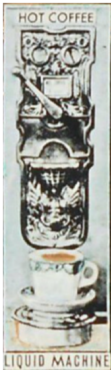
The precise amount of coffee gushed from the mouth of a chrome dolphin's head (copied from a Pompeian fountain) at an exactly calibrated temperature. Image: en.wikipedia.org .
